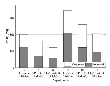
Fig. 3. Testbed experiment results with the limited inter-AS bandwidth: inter-domain traffic (sum of inbound and outbound) related to the Local AS.
