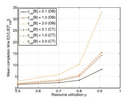
Fig. 5. The completion time for exponentially distributed inter-arrival times of transmission requests is independent of the number of customers n. It depends only for data beaming on the variability of the transmission request sizes.
