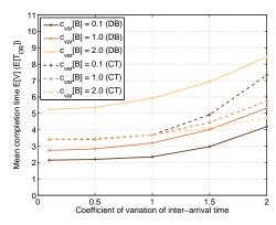
Fig. 6. The completion time for data beaming and concurrent transmission depends on the coefficient of variations  $c_{var}[A]$  and  $c_{var}[B]$  for the request inter-arrival time A by a customer and the request size B ( $\rho = 0.7, n = 100$ ).
