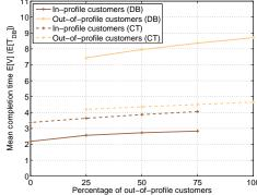
Fig. 8. Data beaming leads to short completion times for in-profile customers and to long completion times for out-of-profile customers while with concurrent transmission the completion time for both customer types does not differ a lot ( $\rho = 0.7, n = 100$ ).
