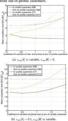
Fig. 7. Completion time for data beaming and concurrent transmission for 50% in-profile and 50% out-of-profile customers with different characteristics ( $\rho = 0.7, n = 100$ ).
