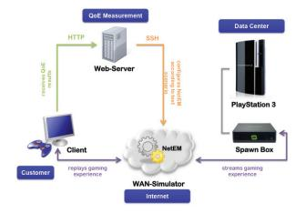
Fig. 1. Testbed Setup - Logical View
