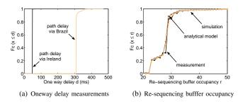
Fig. 1. Measured one way delays and resulting re-sequencing buffer occupancy for measurements, simulation and analysis
