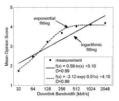
Fig. 5: Web browsing with downlink bandwidth limitation instead of instrumented constant page load times.
