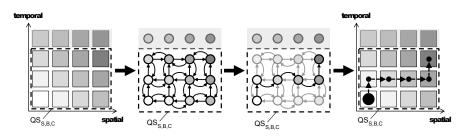
Fig. 2: The steps of interpreting the SVC layer model as graph, retrieving the path with minimal variation from it, and the interpretation as adaptation path.
