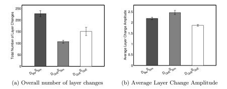
Fig. 5: Layer change characteristics, including the total number of SVC layer changes, and the average change amplitude.
