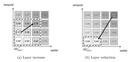
Fig. 1: Examples for  $D_{QoE}$ . The numbers present the QoE ratings based on the Video Quality Metric (VQM).
