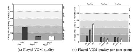
Fig. 6: Comparison of the VQM quality for different adaptation mechanisms.
