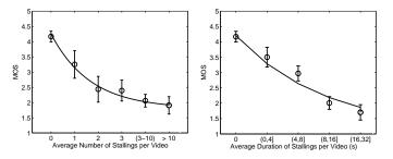
Fig. 3. MOS vs average number (left) and average duration (right) of stallings per video from field measurements.
