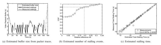
Fig. 4. Estimated stalling patterns from packet traces. Results presented in (b) and (c) correspond to the estimation performed for 100 YouTube videos.
