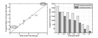
Fig. 6. YouTube QoE real-time monitoring results. (left) Validation with real traces from the field trial. (right) The monitoring is performed at the Gn interface of the 3G HSPA network of a leading European network operator, on a period of 1 hour.
