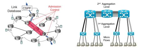
Fig. 3. Link databases allow CSPF computation and AC is performed in the network.
