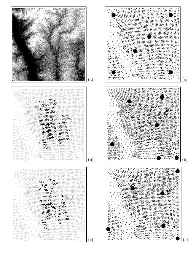
Figure 5: The 3D terrain model (a) and the supplying areas for (b) LOS and (c) ray-tracing
