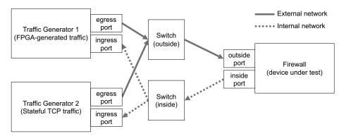
Fig. 1. Hardware setup used in this work.
