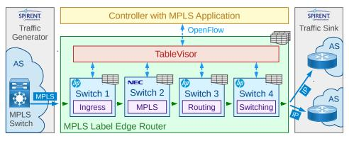
Fig. 5: MPLS Label Edge Routing.
