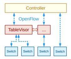
Fig. 6: Vision of an advanced control channel structure with logical TableVisor instances for increased flexibility.
