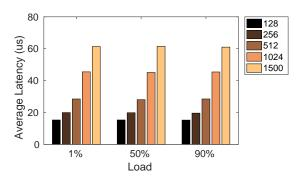
Fig. 3: Data plane delay of an emulated multi-table switch for different frame lengths and load levels.
