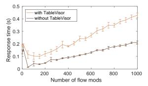
Fig. 4: Setup times for 1 to 1000 flow mods with and without TableVisor.
