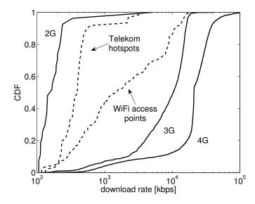
Fig. 1. Throughput of mobile connections for different access technologies.
