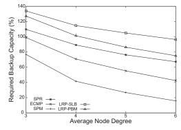
(b) Backup capacity requirements depending on the network connectivity.
