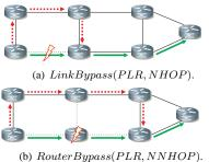
Fig. 2. Facility backup link and router bypasses.
