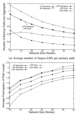
(b) Average prolongation of the path length through bypass-LSPs. Fig. 6. Impact of the network size, the protected failures, and the protection method on the configuration overhead.
