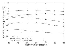
(a) Backup capacity requirements depending on the network size.
