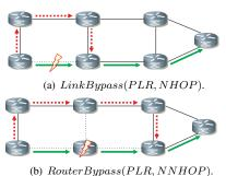
Fig. 3. Facility backup using bypasses.
