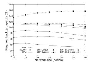
**Figure 8:** Impact of the network size, the protected failures, and the resilience mechanism on the required backup capacity for restoration, end-to-end protection, and local protection.
