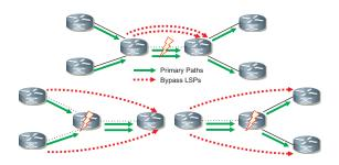
**Figure 6:** In case of router failures the facility backup concept deviates the traffic from and also to different locations in the network, which leads to an even better traffic distribution.
