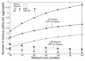
**Figure 7:** Impact of the network size, the protected failures, and the protection method on the configuration overhead.
