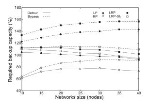
**Figure 4:** Impact of the network size, the protected failures, and the resilience mechanism on the required backup capacity for MPLS-FRR.
