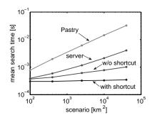
Fig. 4. Mean search time for different network sizes
