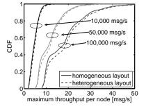
Fig. 6. CDF of maximum message throughput for homogeneous and heterogeneous network layouts.
