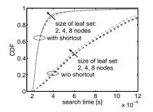
Fig. 5. Comparison of search time distributions for different sizes of the leaf set.
