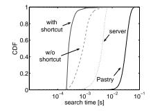
Fig. 2. CDF of the search time for a central server system, an unmodified Pastry, and our modified Pastry both with and without shortcut link.
