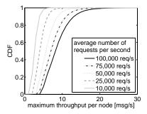
Fig. 7. Maximum number of messages per node in one second
