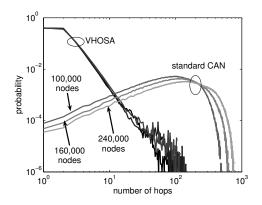
Fig. 3. Hop distribution for a standard CAN network and our modified CAN
