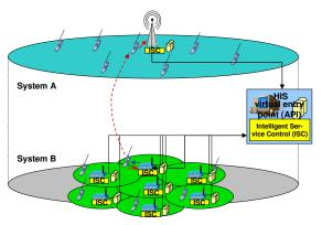
Fig. 1. Distributed information system: the database consisting of measurements is distributed among APs
