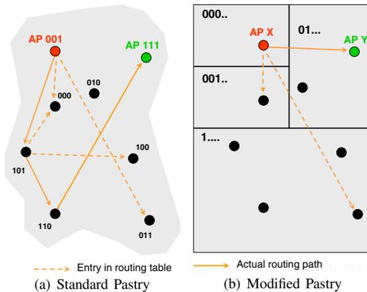
Fig. 3. Routing example with SHA-1 and modified hash function which takes AP location and technology into account
