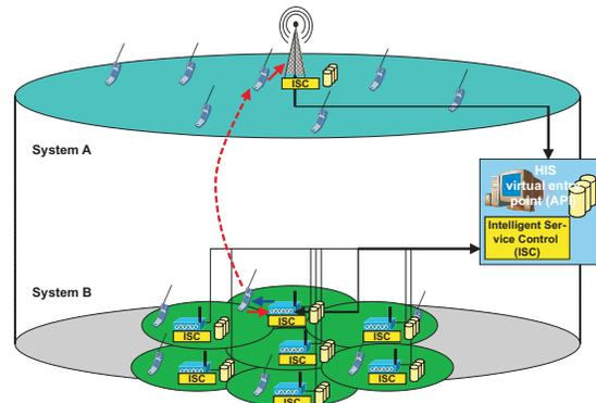
Fig. 1. Distributed information system: the database consisting of measurements is distributed among APs together with the ISC (enhanced figure from [1])
