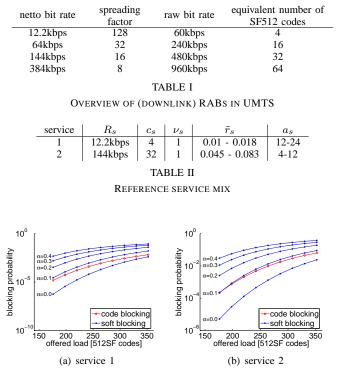
Fig. 3. Impact of orthogonality factor on the relationship of code and soft blocking
