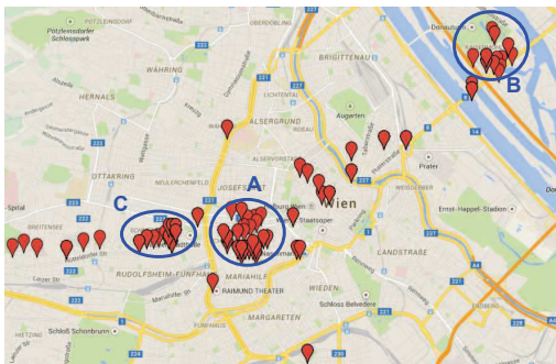
Figure 21. End-device location monitoring and privacy issues. End-user activity and private location can be guessed by simply measuring the location of the cell where smartphone are attached to. In this example scenario, participants’ home is located at region A, working office is located at region B, and high activity occurs at region C, linked to daily train traveling.
