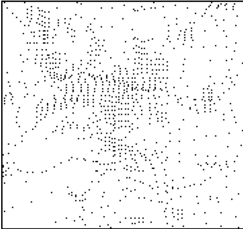
Figure 5.3: Two-dimensional demand node distribution of the Würzburg area generated by partitional clustering
