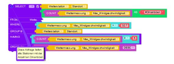
Figure 2: Example of a SQL query with BlocklySQL: It returns the locations of weather stations, where more than five galeforce winds (wind speed > 32.7 m/s) have been recorded (in German). Queries can also be attached with comments and blocks can be collapsed (e.g. FROM-clause) to improve readability.
