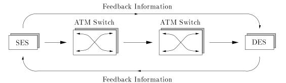
Figure 1: Basic configuration for rate-based congestion control
