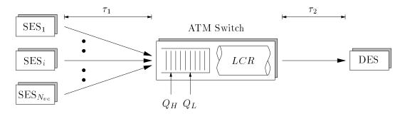
Figure 2: Network model with a single bottleneck link
