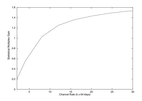
Figure 5: Statistical Multiplex Gain
