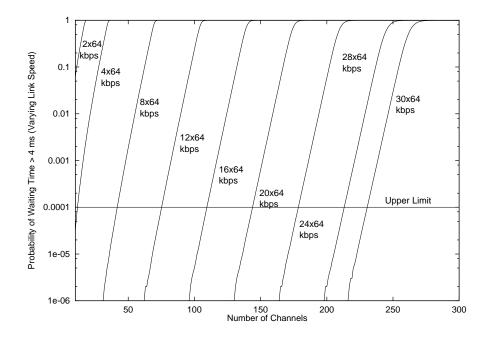
Figure 3: Complementary Packet Delay Distribution
