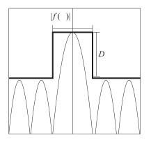
Figure 1: Beam pattern approximation
