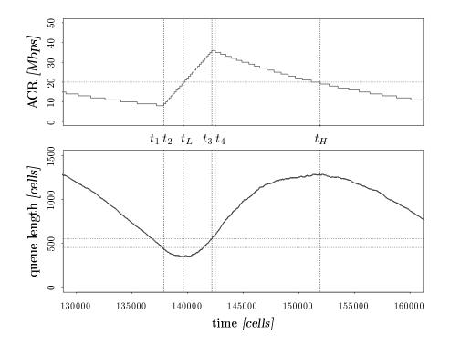
Figure 11: Example evolution for the binary mode of the ABR flow control
