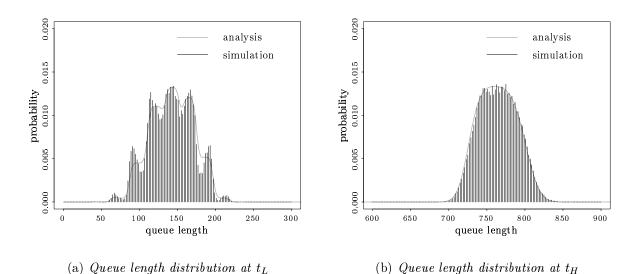
Figure 7: Queue length distributions at the local minimum  $(t_L)$  and maximum  $(t_H)$
