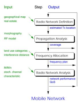
Figure 2: Conventional approach of cellular network planning
