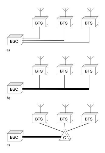
Figure 2: (a) Star, (b) Drop-and-Insert, and (c) Concentrator Architecture
