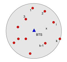
Figure 1: CDMA cell with k supported calls
