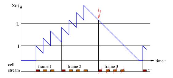
Figure 2: F-GCRA state diagram with three arriving frames.
