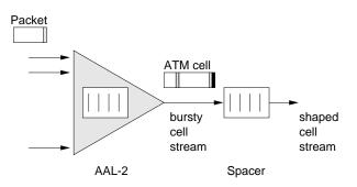
Figure 1: Model of AAL-2 combined with spacer
