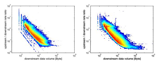
Figure 11: TCP data rate ratio in dependence of downstream data volume for 14.4kbps(left) and ADSL (right).
