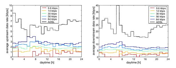
Figure 7: TCP-connection data rate in dependence of daytime.
