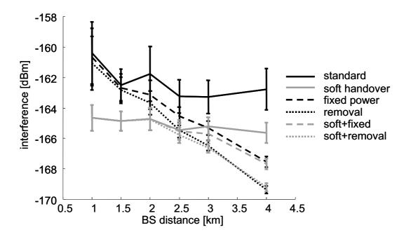
Figure 5: Mean interference depending on the BS distance
