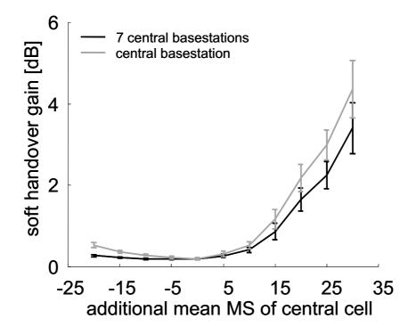
Figure 8: Soft handover gain for inhomogeneous load at central BS
