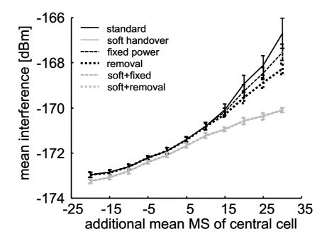
Figure 7: Mean interference for inhomogeneous load at central BS
