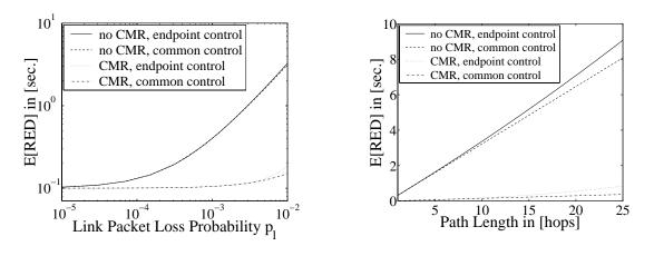
Figure 10: The impact of the control and retransmission option on E[RED] for constant path length.
