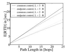
Figure 13: The influence of L and the control option without CMR on E[RED] for high loss rates.
