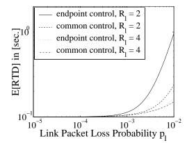
Figure 14: The impact of  $R_l$  and the control option with CMR on E[RED] for constant path length.
