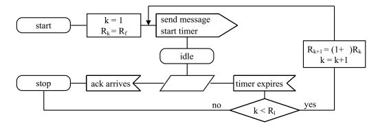
Figure 5: A flowchart of the retransmission algorithm.
