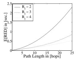
Figure 9: The influence of  $R_l$  with CMR on E[RED] for high loss rates.
