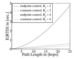
Figure 15: The influence of  $R_l$  and the control option with CMR on E[RED] for high loss rates.
