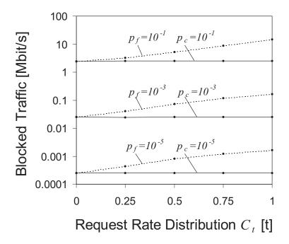
Figure 10: Impact of request rate variability and blocking probability on the blocked traffic.
