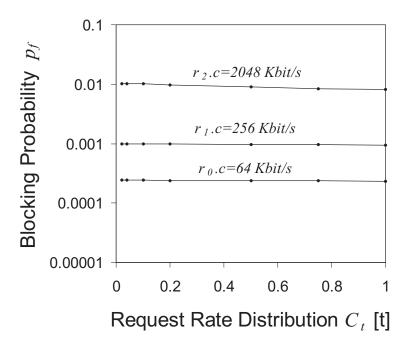
Figure 9: Impact of request rate variability on the rate specific blocking probability for  $p_f = 10^{-3}$ .
