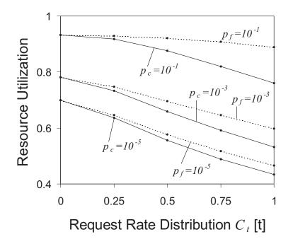
Figure 7: Impact of request rate variability and blocking probability on the resource utilization.
