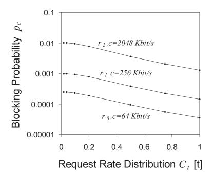
Figure 8: Impact of request rate variability on the rate specific blocking probability for  $p_c = 10^{-3}$ .
