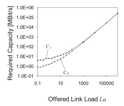
Figure 4: Impact of offered load and request rate variability on the required link capacity.
