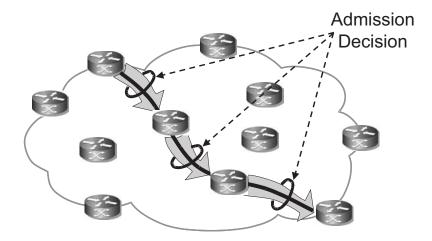
Figure 1: Network admission control based on link budgets.
