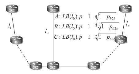
Figure 12: The setting of the link blocking probabilities has a large impact on  $LB(l_0).p$ .
