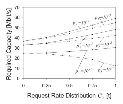
Figure 11: Impact of request rate variability and blocking probability on the required capacity.
