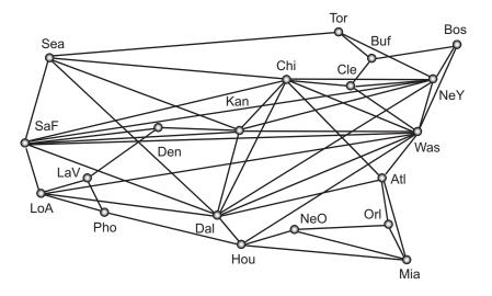
Figure 14: Test network based on the UUNET (1994).
