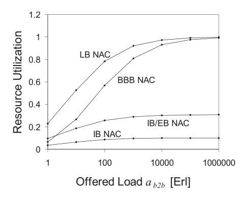
Figure 16: Impact of the offered load and the NAC method on the resource utilization.
