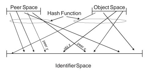
Figure 1: Distributing peers and documents into the identifier space using a hash function
