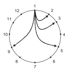
Figure 3: Finger-table of peer 1 in a 12 peer Chord ring
