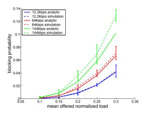
Fig. 4. Blocking probabilities for three service classes
