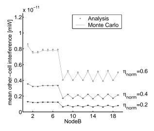
Fig. 2. Mean other-cell interferences in a hexagonal cell layout
