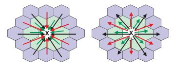
Fig. 1. Interference originating from and coming to NodeB x
