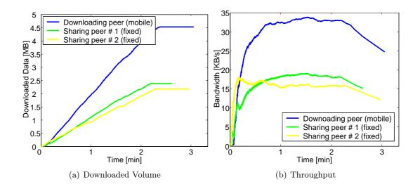
Figure 11: Multiple Source Download in UMTS (mobile:fixed/fixed)
