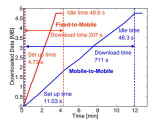
Figure 14: Setup and download times for UMTS (mp3 file)
