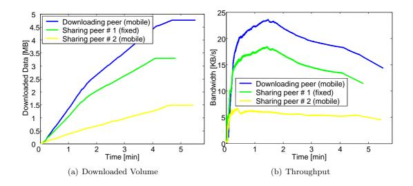
Figure 12: Multiple Source Download in UMTS (mobile:fixed/mobile)
