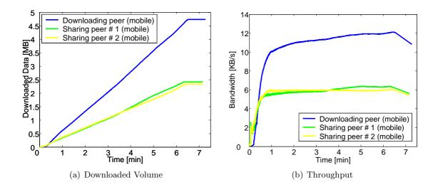
Figure 13: Multiple Source Download in UMTS (mobile:mobile/mobile)
