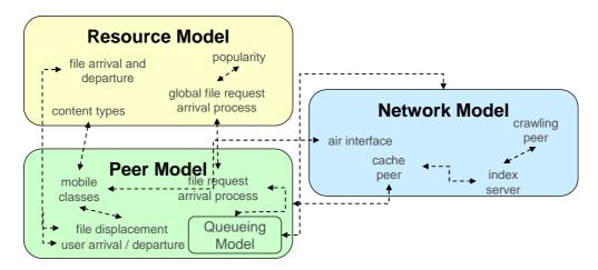
Figure 2: Components of the mobile P2P simulation model
