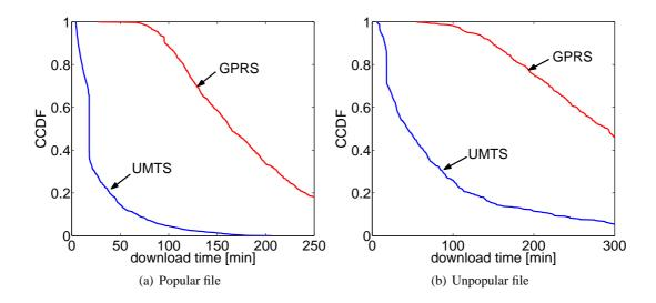
Figure 7: Download of mp3-audio files with GPRS and UMTS
