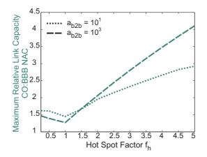
Figure 9: Impact of the overload on the maximum additional relative link capacity requirements.
