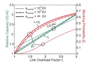
Figure 5: Impact of rare overload on capacity requirements and blocking.
