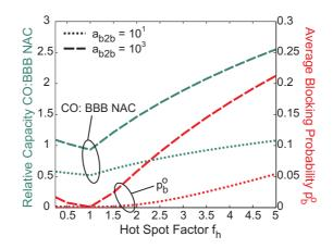
Figure 8: Impact of the hot spot factor  $f_h$  on capacity requirements and blocking.
