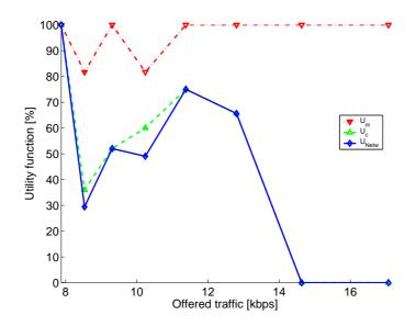
Figure 5: Utility functions versus  $U_{\text{Netw}}$ ,  $U_m$  and  $U_c$  versus offered traffic  $o_A$  in the GPRS uplink case.
