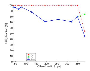
Figure 2: Utility functions  $U_{\text{Netw}}$ ,  $U_m$  and  $U_c$  versus offered traffic  $o_A$  in the UMTS downlink case.
