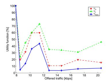
Figure 3: Utility functions  $U_{\text{Netw}}$ ,  $U_m$  and  $U_c$  versus offered traffic  $o_A$  in the GPRS downlink case.
