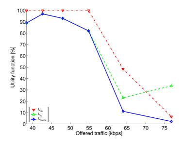
Figure 4: Utility functions versus  $U_{\text{Netw}}$ ,  $U_m$  and  $U_c$  versus offered traffic  $o_A$  in the UMTS uplink case.
