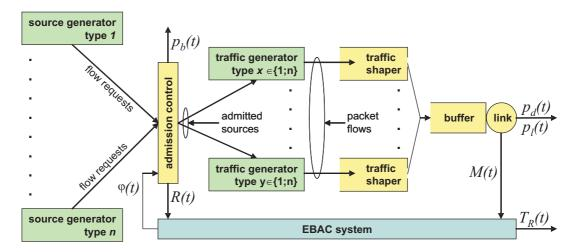
Figure 1: Simulation design for EBAC in steady and transient state.
