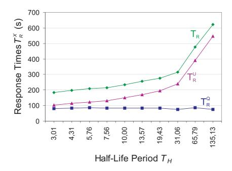
Figure 6: Correlation of EBAC memory with half-life period  $T_H$  and EBAC response times  $T_R^X$  for increasing traffic intensity.
