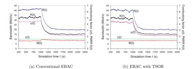
Figure 5: Overbooking performance of conventional EBAC vs. EBAC with TSOB during a traffic intensity increase.
