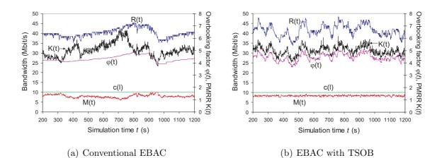
Figure 3: Overbooking performance of conventional EBAC vs. EBAC with TSOB for a constant traffic mix.
