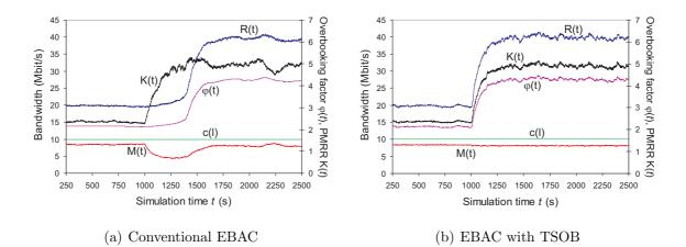
Figure 4: Overbooking performance of conventional EBAC vs. EBAC with TSOB during a traffic intensity decrease.
