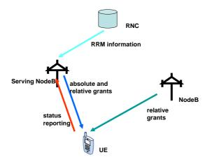
Figure 1: Overview of the rate control functionality of the E-DCH
