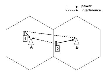
Figure 4: Simple example scenario with two mobiles
