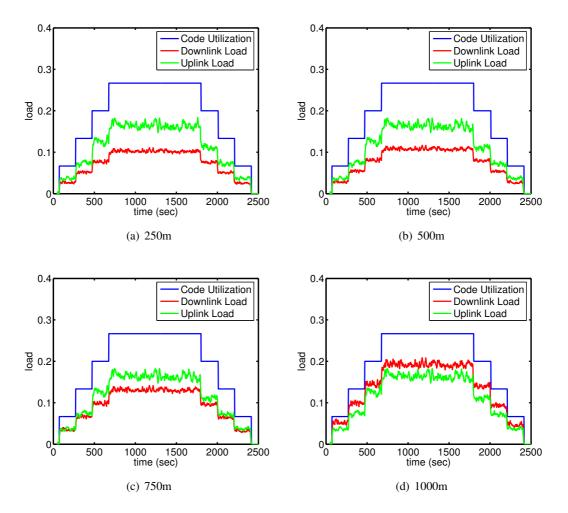
Figure 4: Uplink Load, Downlink Load, and Code Utilization for the following distances to the NodeB: (a) 250m,(b) 500m,(c) 750m, and(d) 1000m.
