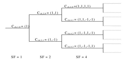
Figure 1: Orthogonal variable spreading factor code tree
