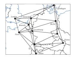
Figure 5: Topology of the COST239 network.
