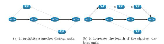
Figure 2: Impact of the wrong selection of the first shortest path.
