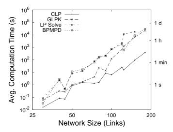
Figure 6: Average computation time of the GLPK, BPMPD, CLP, and LPSolve for the optimization of different random networks depending on the network size in links only.
