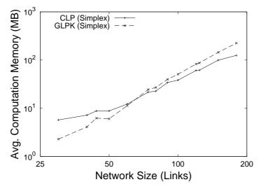
Figure 7: Average memory consumption of the CLP and GLPK solvers for the optimization of different random networks depending on the network size in links only.
