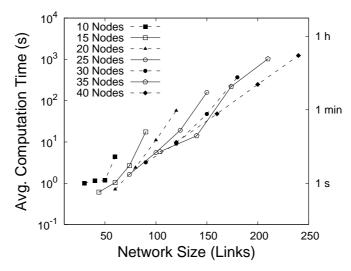
Figure 8: Average computation time of the CLP for the optimization of different random networks depending on the network size in links and nodes.
