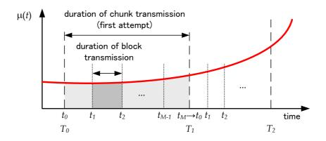
Figure 2: Computation of block and chunk transmission durations from  $\mu(t)$
