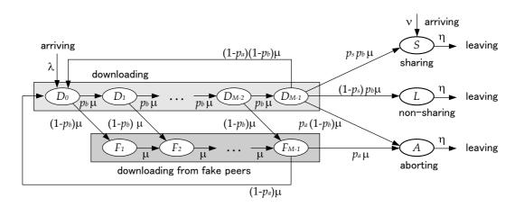
Figure 1: Flow diagram of P2P file sharing model
