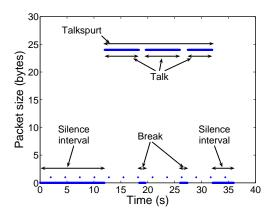
Figure 1: G.723.1 outputs an audio stream and control information. The audio stream consists of silence intervals and main talkspurts that are interrupted by short breaks and noise.
