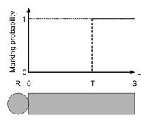
Figure 1: The threshold marker marks packets if the length of its virtual queue exceeds its threshold T.
