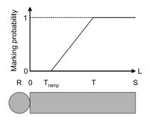
Figure 2: The ramp marker marks all packets if the length of its virtual queue exceeds its threshold T, but it also marks packets probabilistically between  $T_{ramp}$  and T.
