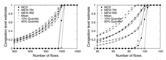
(c) Increased aggregation level: capacity for n = 1000 (d) Increased inter-arrival time variation:  $c_{var}[A] =$  flows instead of n = 100 flows. 1.0 instead of  $c_{var}[A] = 0.1$ .
