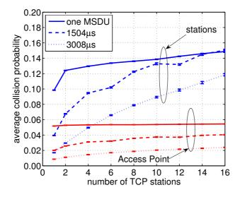
Figure 6: Impact of transmission bursts on the collision probabilities
