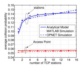
Figure 4: Unfairness between AP and stations using saturated TCP traffic on the downlink
