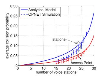
Figure 3: Comparison of OPNET simulation results with the complete DCF and analytical results
